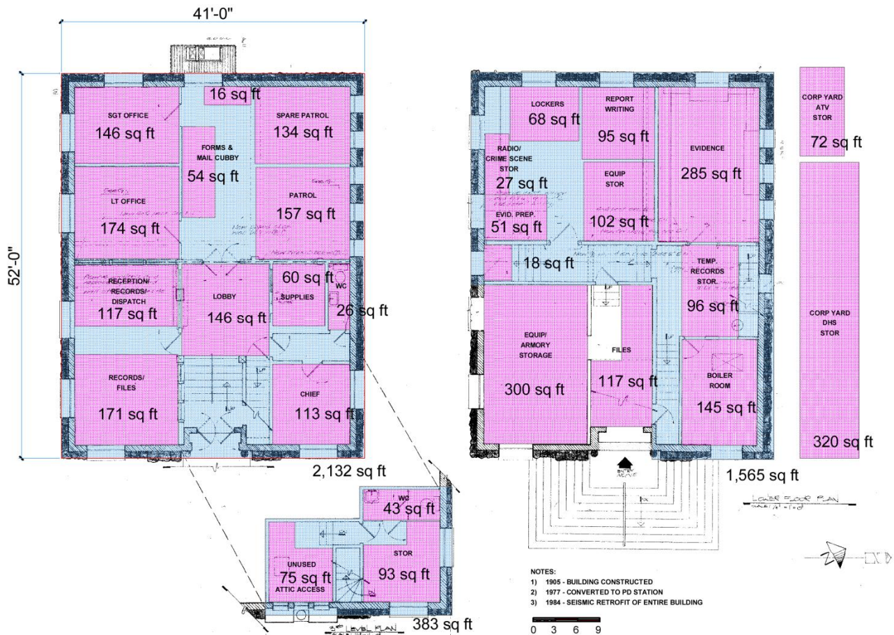
Figure 41 - Plans of Existing Police Space
